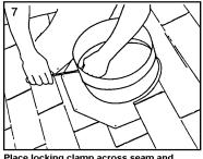
Place locking clamp across seam and tighten with machine screw.
